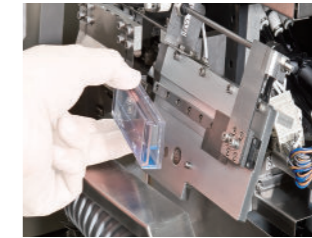
Installation of the cassette
